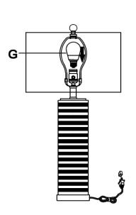
Step2 Insert the bulb(G) into the socket(C).
