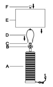
Step 1 Insert the Harp (D) into the Saddle (B). Put the shade(E) on the Harp(D), then tighten the Finial (F)into the Harp (D)
