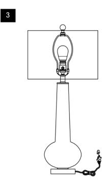
Step2 Insert the bulb( G) into the socket(C).
