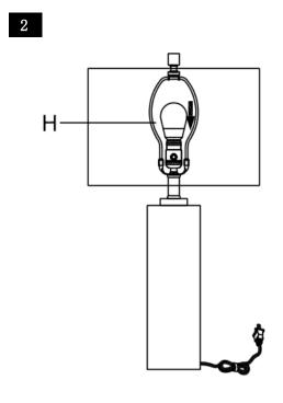
Step2 Insert the bulb( H) into the socket(C).
