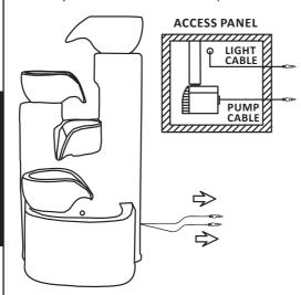
**3.** Fill the reservoir with water, ensuring the pump will remain fully submerged during operation.
