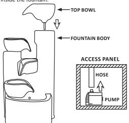
**2.** Extend the pump and LED light cables through the access hole in the back of the fountain, cables are ready for connection to the solar panel.
