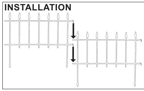
Assistance may be required to ensure the panels remain linked during installation.
