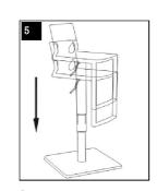
Step 4 Place the assembled seat onto the base and make sure it is placed vertically.
