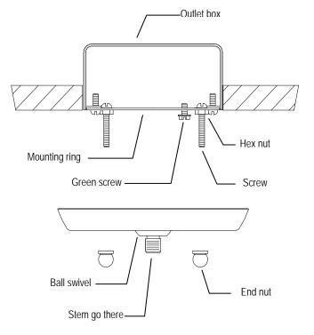
5. Fasten the ribbed fixture lead to white wire or ribbed wire in the outlet box. Fasten the wires together with an approved fastener (wire nut). Starting about 1" below the fastener, Tightly wrap the connection with electrical tape so that the connection seals the end of the fastener.
