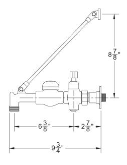
**General:** Chrome plated brass service sink faucet, ½" pipe eccentric inlets on 8" centers. Vacuum breaker integral stops, chrome plated (H&C) handles, ¾" hose end spout with pail hook, top reinforcing bar and mounting bracket. Install as shown on plans and in accordance with local codes.
