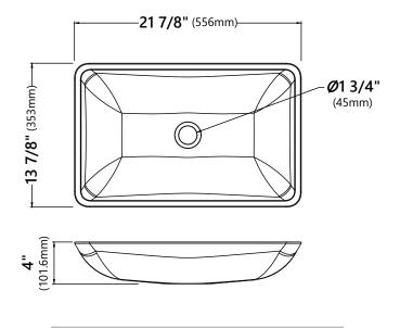
Model #: GVR-204-RE, GVR-210-RE Sink Dimensions: 21 7/8" x 13 7/8" x 4" Glass Thickness: 15mm
