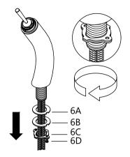
Remove mounting hardware (6A, B, C, & D) from the mounting pipe.
