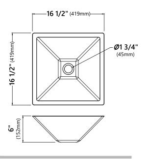
Model #: GVS-901-19mm Sink Dimensions: 16 1/2" x 16 1/2" x 6" Glass Thickness: 19mm
