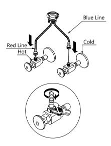
Connect hot and cold waterlines (7) to the angle stops. Tighten with a wrench until snug. Turn on hot and cold angle stops and check for leaks.
