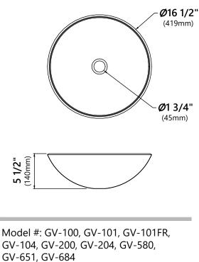
Sink Dimensions: Ø16 1/2" x 5 1/2" Glass Thickness: 12mm
