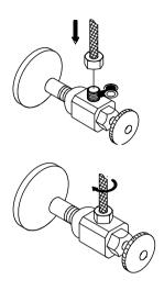
Install flex water supply lines on the angle stops and tighten with an adjustable wrench. Turn on both the cold and hot main valves Apply pipe tape (optional).
