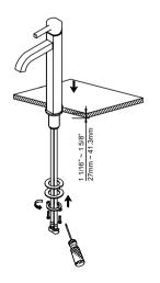
Install the faucet through the 1-3/8" predrilled hole in the countertop. Attach rubber washer (4A), metal washer (4B), mounting nut (4C), and mounting screws (4D) on the threaded mounting pipe. Tighten the mounting nut (4C) until snug. Tighten screws (4D) on the mounting nut (4C) with a Phillips head screwdriver until snug.
