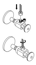
Install flex water supply lines on the angle stops and tighten with an adjustable wrench. Turn on both the cold and hot main valves Apply pipe tape (optional).
