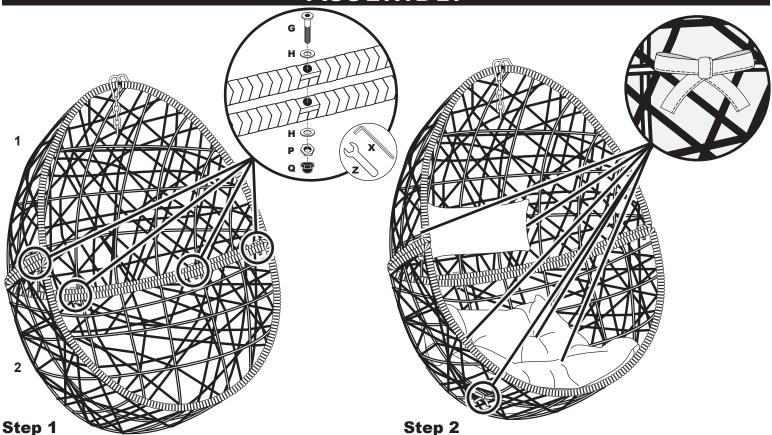
Align Chair Top (1) and Chair Bottom (2) and secure them using Bolt (G), Washers (H), and Lock Nut (P). Place Hex Nut Cap (Q) over the lock nut.
