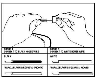
**A.** Take note of the color of the wire(s) on your fixture. Identify which group your fixture wire(s) falls into and connect the wires according to the directions below:
