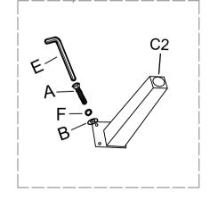
Do not fully tighten until all bolts have been inserted.
