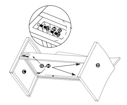
Secure the Side Panels to the Backrest ③. Place a Washer ① on each of 4 Bolts ③. Insert a Bolt with Washer through each of the 4 aligned sets of eyelets.
