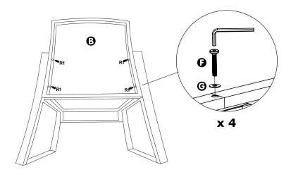
Turn assembled chair upright on a flat, level surface to ensure that it sits squarely and level on the ground. Adjust fastenings if needed, then firmly tighten all **Bolts** installed in Steps 1–3.
