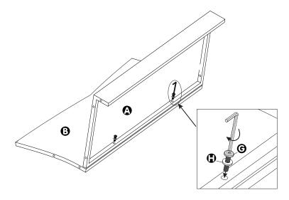
Attach the Left and Right Panels ( ) to the assembled seat: Place a Washer ( on each of 6 Bolts ( ). Align the eyelets on the Left Panel with the holes in the edge of the Seat Panel as shown, then insert a Bolt with Washer into each of the 3 aligned sets of eyelets (1 behind the front panel of the seat, 2 along the side of the seat). Gently tighten using Hex Wrench without fully tightening. Repeat to attach the Right Panel.
