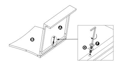
Attach the Left and Right Panels ( ) to the assembled seat: Place a Washer ( on each of 6 Bolts ( ). Align the eyelets on the Left Panel with the holes in the edge of the Seat Panel as shown, then insert a Bolt with Washer into each of the 3 aligned sets of eyelets (1 behind the front panel of the seat, 2 along the side of the seat). Gently tighten using Hex Wrench without fully tightening. Repeat to attach the Right Panel.
