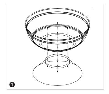
Attach Handle (A) to Fire Screen (B) with a Nut (1). Securely tighten.
