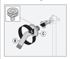
5) Install showerhead (A) to shower arm (B). Turn clockwise to tighten.
