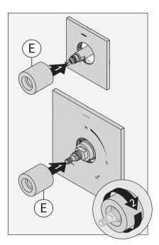
5) Install diverter handle (3605 and 3606 only) (D) and shower handle (D) to valves. Secure handles by tightening set screws.
