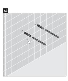
Please note if the washbasin will be mounted on a concrete wall application, anchors must be used.
