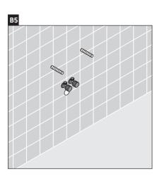
Install Shut off valves according > to manufacturer's installation instructions.
