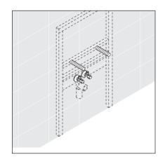
When mounting the washbasin on a pre-wall carrier, install the mounting bolts to the element.
