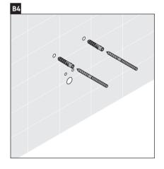
Please note if the washbasin will be mounted on a concrete wall application, anchors must be used.
