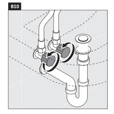
Turn on Shut off valves to test water flow to faucet and drain. >
