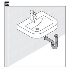
Install the siphon according to the corresponding installation instructions.
