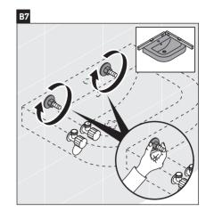
> Leveling the washbasin: the white plastic sleeves protect the china from the metal bolt and allow for slight adjustment in the height of the washbasin to level it.
