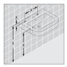
The washbasin specification sheet will provide the recommended mounting height and show the location of the mounting holes. (The height can be adjusted to your personal preference)
