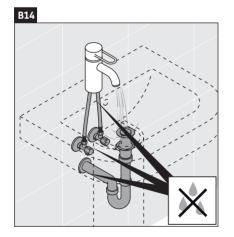
> Test faucet and drain to ensure there are no leaks.
