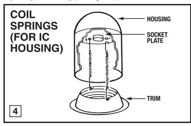
**FOR 1154 TRIMS / EYEBALL TRIMS:** Before installing trim, remove socket plate from housing by loosening wing nut. Unfasten socket from socket plate by squeezing springs and snap into hole provided in top of trim (see Diagram 5). If using 1155ATR (See Diagram 5). Discard socket plate / bracket.
