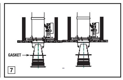
**TO INSTALL LAMPS:** Select proper lamp (see lamp maximum wattage label in housing). Do not exceed maximum wattage lamp shown for each trim.
